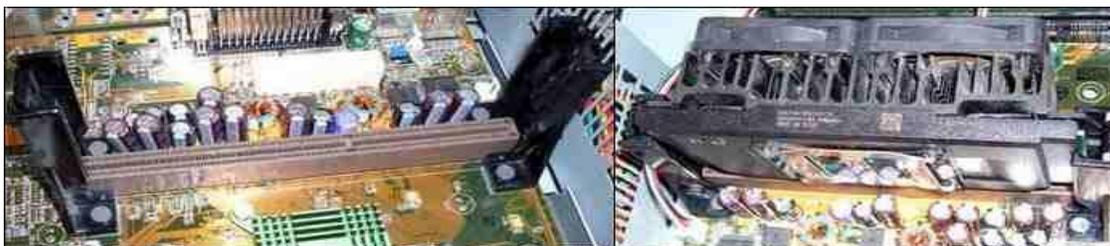
Slot 1 connector is 5.23" long (13.29 cm). Besides the actual connector, the Slot 1 also includes SEC cartridge retention mechanism required to support a processor in SEC cartridge and a heatsink. Maximum supported weight of the processor with the heatsink is 400 grams.
