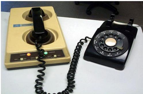
The early modems were acoustic and connected directly to the handset of a telephone. The modem had acoustic insulation around both the mouthpiece and earpiece of the handset to reduce outside noise.
