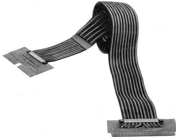
**Figure: The Unibus of the PDP-11 Computer**
