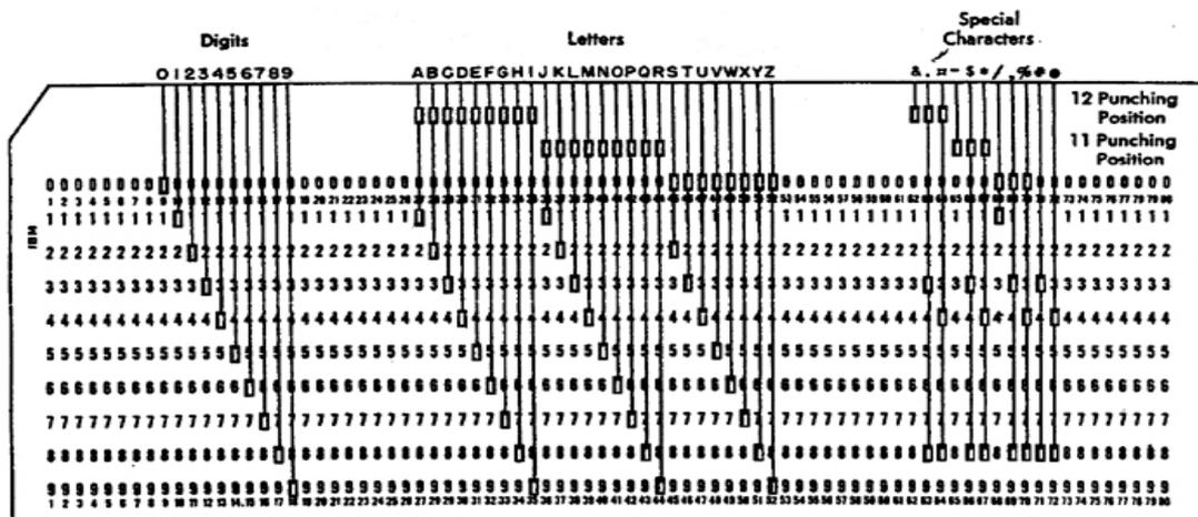
Note the structure of the column punches for the alphabetic character set. Each letter is represented by a punch in either column 11 or 12 (the zone punch) and a punch in one of the columns numbered 0 through 9 (the numeric punch). While the digits are represented by a single punch, the requirement to have a full-byte representation in the character code has lead to their being assigned a zone code as well.
