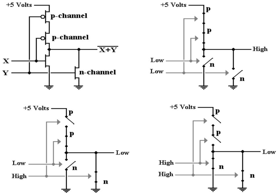
Note that the output is high (logic 1) only when both of the inputs are low (logic 0). If either input is high (logic 1), then the output is low (logic 0). This is a NOR gate.
