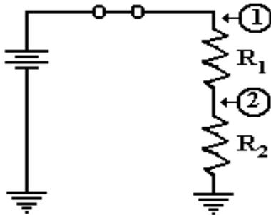
In general,  $E_2 = (E \cdot R_2) / (R_1 + R_2)$ , the value being somewhere between the full voltage and ground voltage, defined to be zero.
