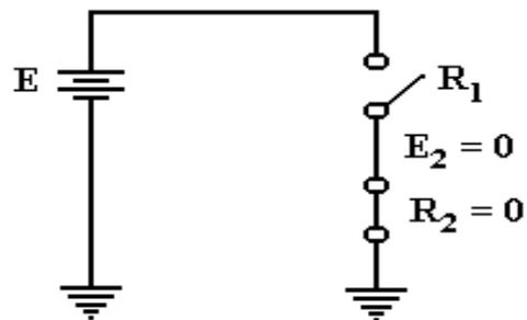
When the top switch is closed ( $R_1 = 0$ ) and the bottom switch is open ( $R_2 \neq 0$ ), the voltage  $E_2$  is the full voltage. When the top is open and the bottom closed,  $E_2 = 0$ .
