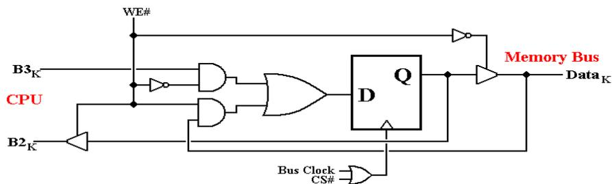
First consider the connection of the output of the flip-flop in the MBR.
