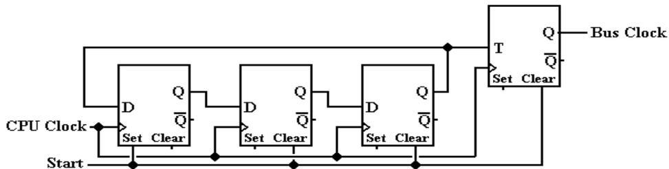
This is a one-hot modulo-3 counter. On every third pulse, the input to the T flip-flop is set to 1 and that flip-flop toggles. The bus clock output from the T has frequency 1/3 of the CPU clock. All that is generally true is the CPU clock frequency is some integer multiple of the bus clock frequency, as the bus clock is derived from the CPU clock by methods similar to that above.
