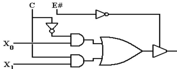
When  $E\# = 0$ , the output of the multiplexer depends on the value of the control signal,  $C$ . When  $E\# = 1$ , the OR gate of the multiplexer is disconnected from the output.
