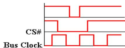
The diagram at left shows the timing of the control signals. The signal  $CS\#$  is asserted as 0 some time during the high phase of the bus clock and remains low until some time in the next high phase. The clock signal to the flip-flop has a well defined negative edge, allowing it to be loaded properly.
