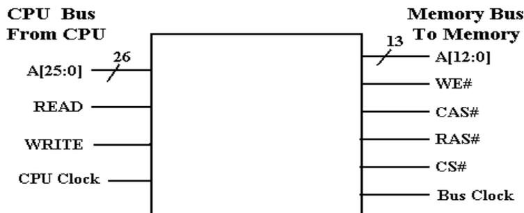
Immediately, we can derive equations for WE# and CS#, assuming that there is only one chip. In actual fact there will be more than one memory chip, but the CS# developed here will be an input to the values sent to each of the multiple chips.
