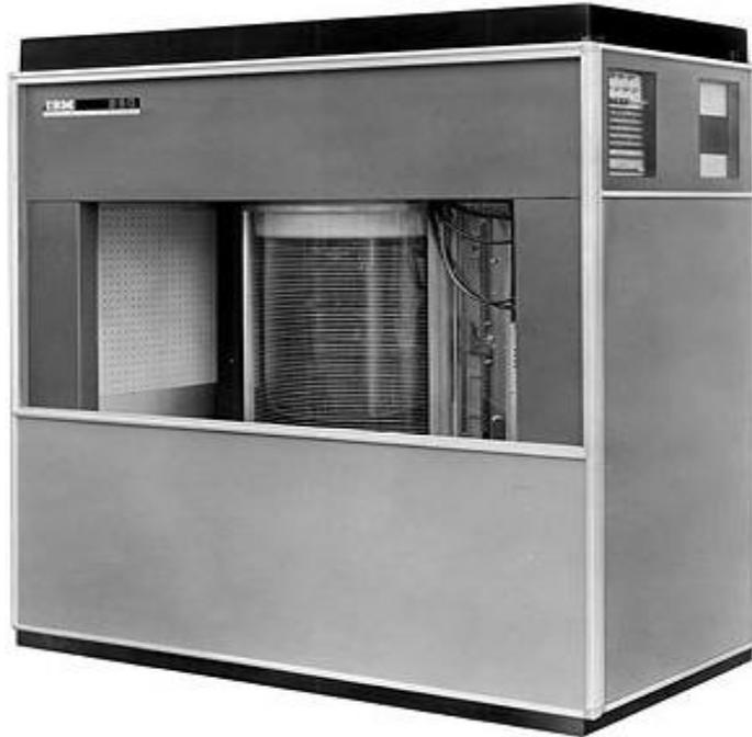
**Figure: The Disks of the RAMAC 305**
