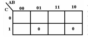
This is really somewhat of a trick question used only to illustrate placing of the terms for POS. Place a 0 at each location, rather than the 1 placed for SOP. Note that the two 0's placed are not adjacent, so we cannot simplify the expression.
