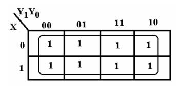
The sample at left, based on an earlier design shows a particularly simple problem. We find that all the entries in the K-Map are covered with a single grouping, thus removing all three variables. Since the entire K-Map is covered, the simplification is F = 1.
