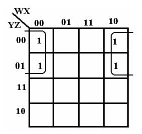
The first row in the K-Map represents the entries 0000 and 1000. The second row in the K-Map represents the entries 0001 and 1001. The trick here is to see that the last column is adjacent to the first column The four cells in the K-Map are thus adjacent and can be grouped into a square. We simplify by noting the values that are constant in the square: X = 0 and Y = 0. Thus, the expression simplifies to X'•Y', as required.
