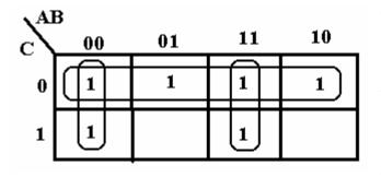
The top row of the K-Map corresponds to the entries 000, 010, 100, and 110, arranged in the order 000, 010, 110, and 100 to preserver logical adjacency. The bottom row corresponds to the entries 001 and 111. The top row simplifies to C'. The first column simplifies to A'B' and the third column to AB. Thus we have  $F(A, B, C) = A' \cdot B' + A \cdot B + C'$ . We next consider a somewhat offbeat example not in a canonical form.
