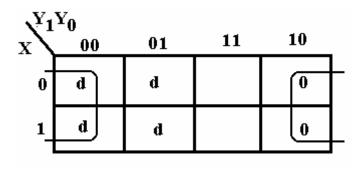
The POS simplification is shown at left. The top row simplifies to 0-0 and the bottom row simplifies to 1-0 so the K-Map simplifies to -0. Using the POS copy rule, this translates to Y<sub>0</sub>, as before. It's a good thing that the two methods agree.
