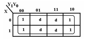
The sample at left, based on an earlier design shows a particularly simple problem. We find that using the d's to combine with the 1's to produce a 4-by-2 grouping of 1's. Since the entire K-Map is covered, the simplification is F = 1.
