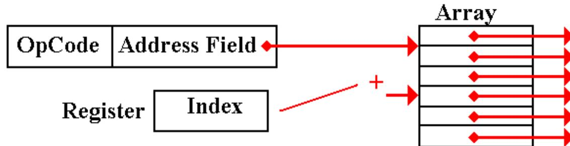
**Post-Indexed Indirect:** The indirect is done first. We have a pointer to an array.
