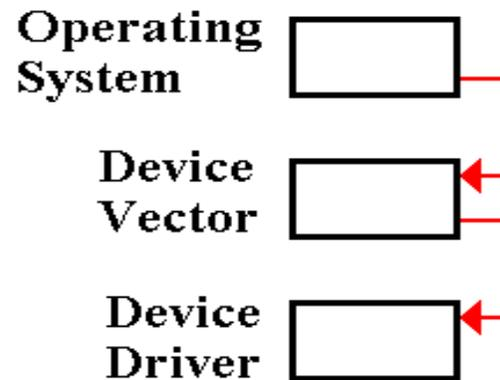
This arrangement allows the operating system and the device drivers to be developed independently. The only fixed location is the address of this device vector.
