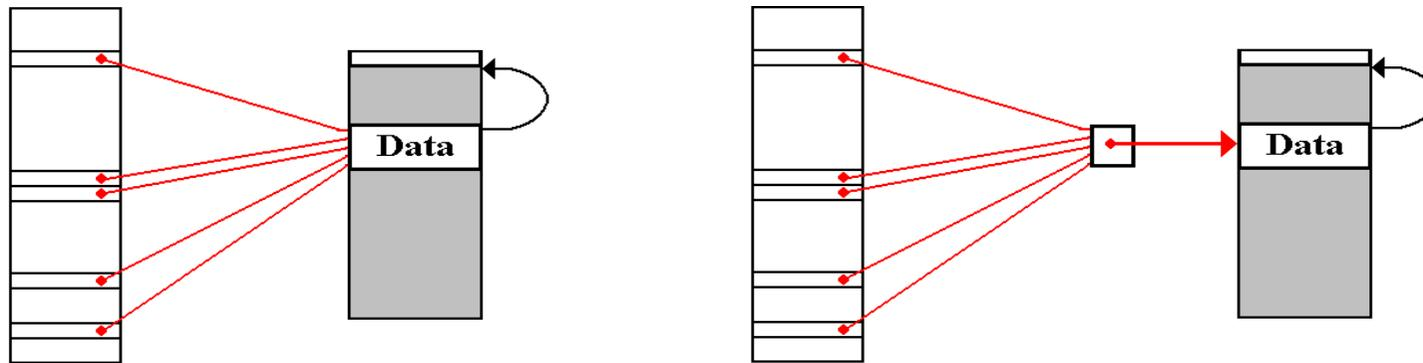
Singly indirect addressing, in which the pointer is stored in every program, presents problems when the data block is moved by the memory manager. Every reference to that block must be found and adjusted.
