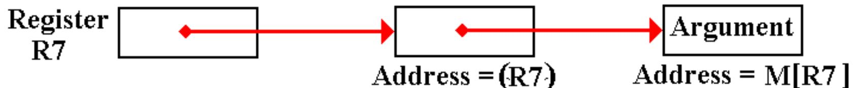
We would have to make the control unit more complex to remove this addressing mode.
