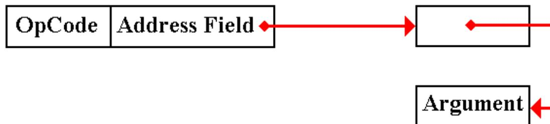
In subroutine linkage, argument passing by preference basically uses indirect addressing.
