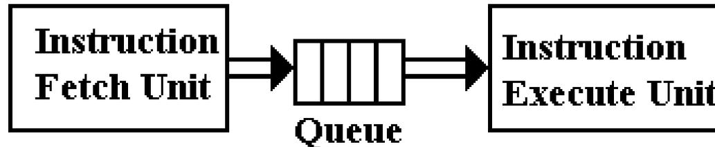
Here we assume that the prefetch unit maintains a queue of instructions that are ready to be run by the execution unit and immediately available for transfer to the IR.
