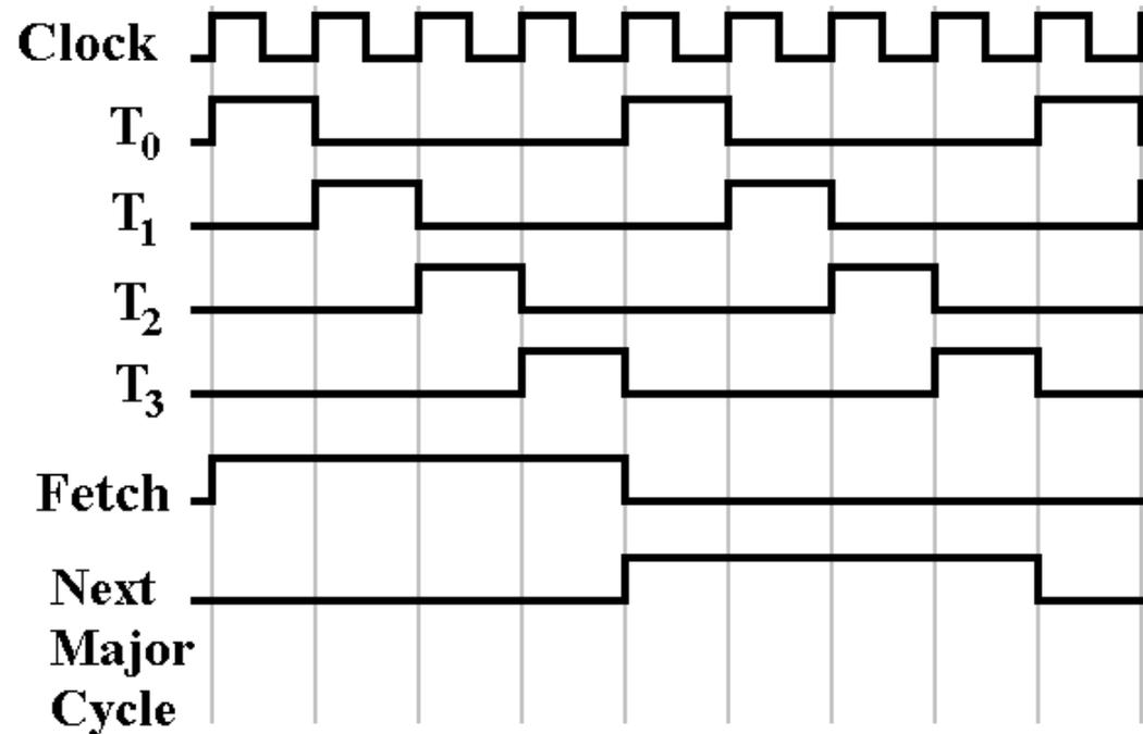
Here we see that each minor state is active for exactly the duration of one clock pulse.
