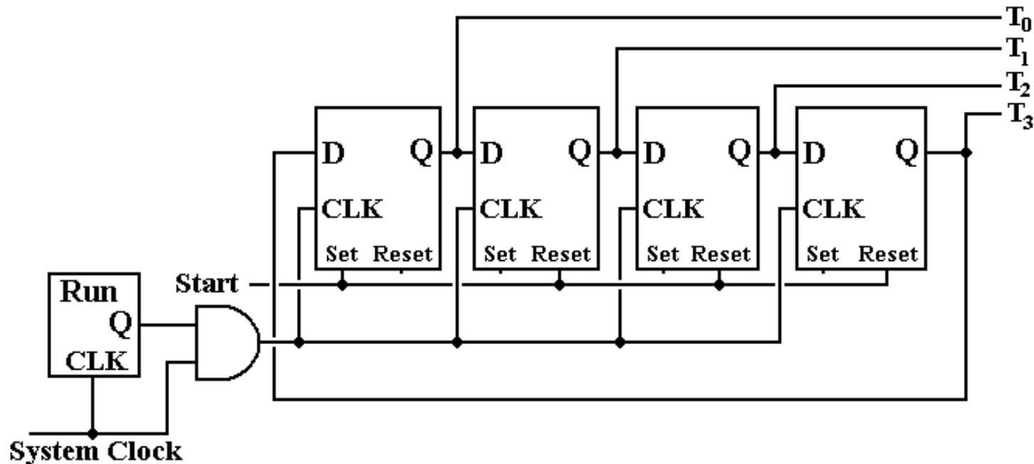
When the run flip-flop is set, the clock pulses get through to the state register and cause it to count.
