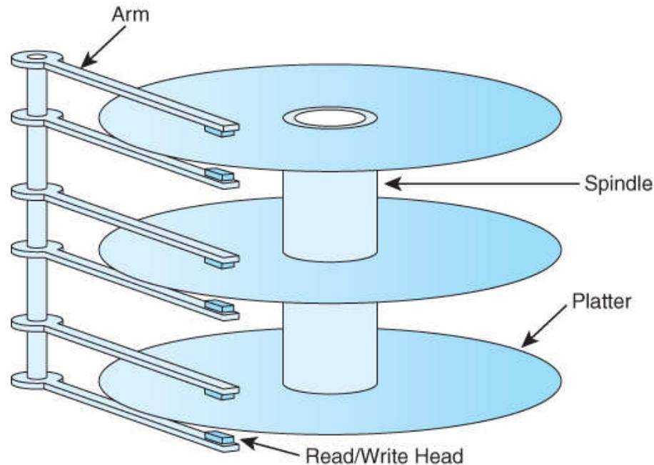
This drawing shows a disk with three platters and six surfaces. In general, a disk drive with  $N$  platters will have  $2 \cdot N$  surfaces, the top and bottom of each platter.
