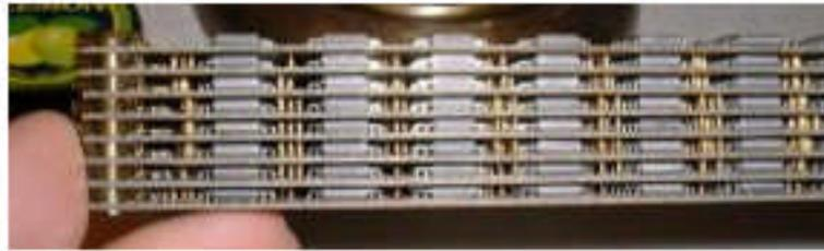
Due to the card density, it was not possible to use air cooling. The entire system was immersed in a tank of Fluorinert™, an inert liquid intended to be a blood substitute.
